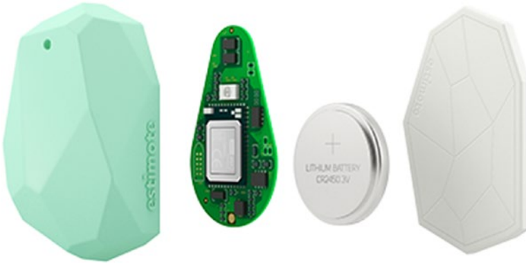
Figure 4-9. A deconstructed Bluetooth beacon
